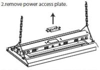
4.Power input from side: Remove knockout inendcap and install 1/2\*conduit, or B) install AC power cord with strain relief. Plug unused hole on power access plate with appropriate fitting
